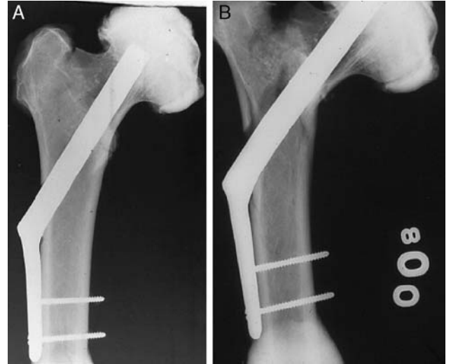
FIGURE 6. Cadaver bone with an artificially produced high intertrochanteric fracture nailed with a 150° angle nail. Collapse of the fracture occurred when 800 pounds of vertical load was applied, a load several times greater than the intrinsic strength of the nail.
